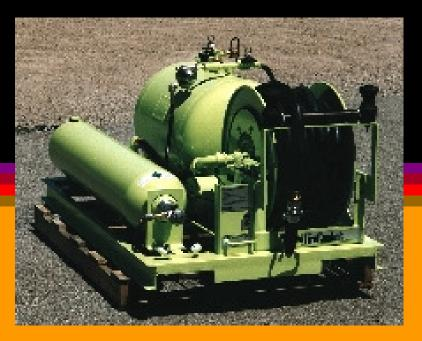
Mounted on pickup bed or trailer, Halotron/I can be quickly moved to quench fires. It can also be mounted on skid to give on-site protection for aircraft hangars, offshore platforms, turbine/generator sets, and transformer vaults. Rig has 300 cu. ft cylinder carrying compressed argon and 460 lb Halotron-filled tank. In operation, pressurized argon spews out Halotron at 225 psi, effectively smothering fire. It meets EPA and FAA requirements.
